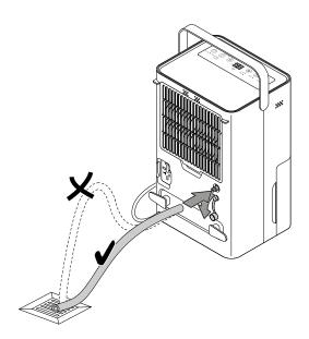
4. Remove the hose if you want to collect the condensate in the condensation tank again. Allow the hose to dry prior to storage.
