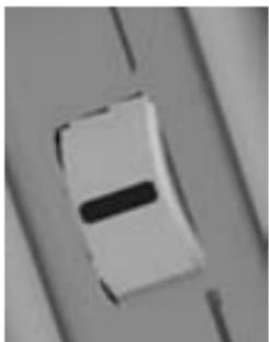
In contrast to conventional hand-held measuring devices this measuring device does not have a keypad but what is known as a "THUMB-WHEEL" on the left-hand side of the device.
