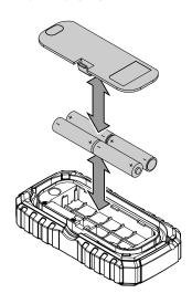
3. Put the cover back onto the battery compartment.
