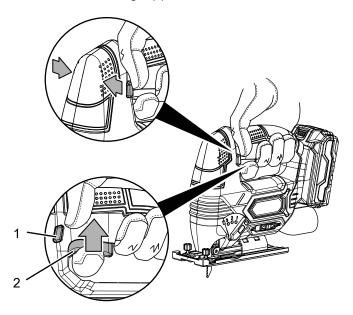
6. Let go of the on-/off-switch (2) to stop the device.
